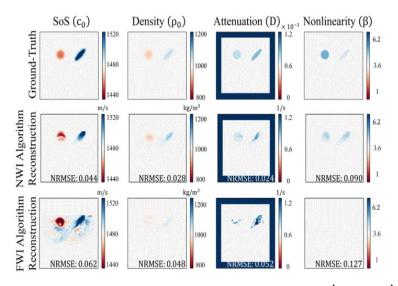
Reconstruction of simulated medium properties (headers), using the NWI algorithm compared to the FWI. The left and right objects are fat and liver, respectively.
