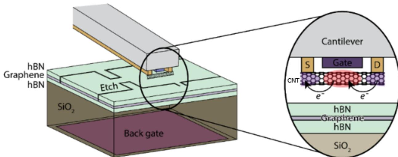
A schematic presentation of the arrangement of the carbon nanotube on the SET detection arm. The nanotube is connected to source and drain electrodes (yellow) and suspended above multiple gates (blue). The CNT structure is designed to scan the device of interest with no charge directly transferred between the probe and the inspected area.
