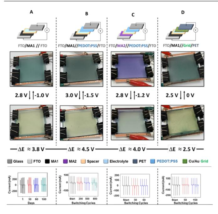
Electrochromic devices (ECDs) bearing a surface area of 6 X 6 cm. Top: Schematic presentation of the ECDs based on working electrodes. Middle: Photographs of the colored and bleached states of the ECDs C. Bottom: Chronoamperometric stability measurements.
