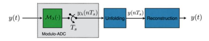
A schematic of modulo-sampling and reconstruction
