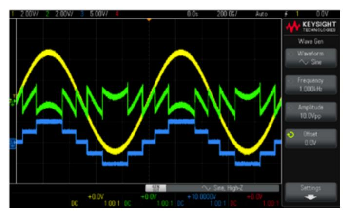
Oscilloscope screenshot showing 1† $\bar{k}$ Hz sinusoid (yellow), modulo-folded output (green), and DVG signal (blue) with peak amplitude of  $4\hat{l}$ »
